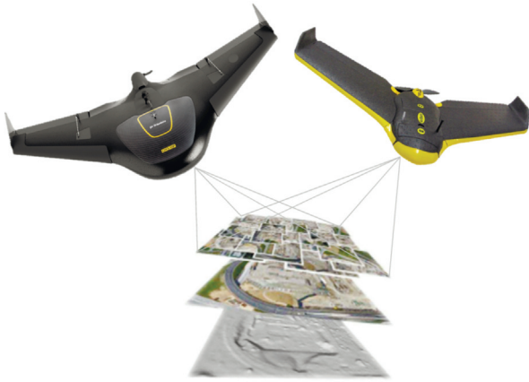
Fig. 4 Drone Trimble UX5 and Sensefly eBee collecting data
