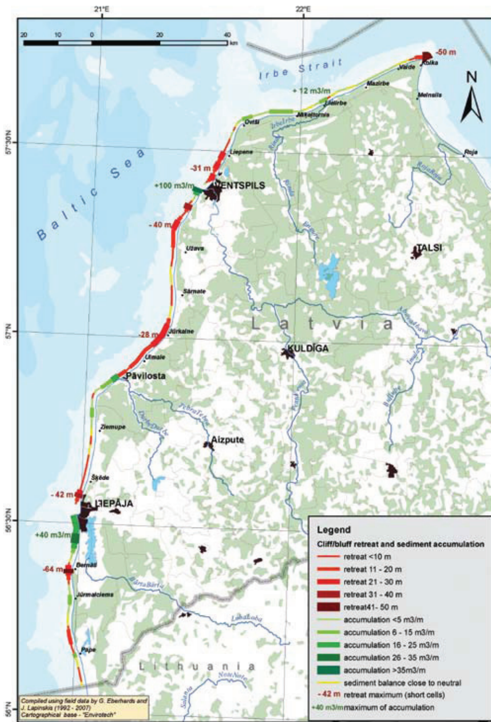
Fig. 4. Changes to the Kurzeme coast of the Baltic Proper during the past 15 years (1992–2007). Compiled by G. Eberhards and J. Lapinskis.
