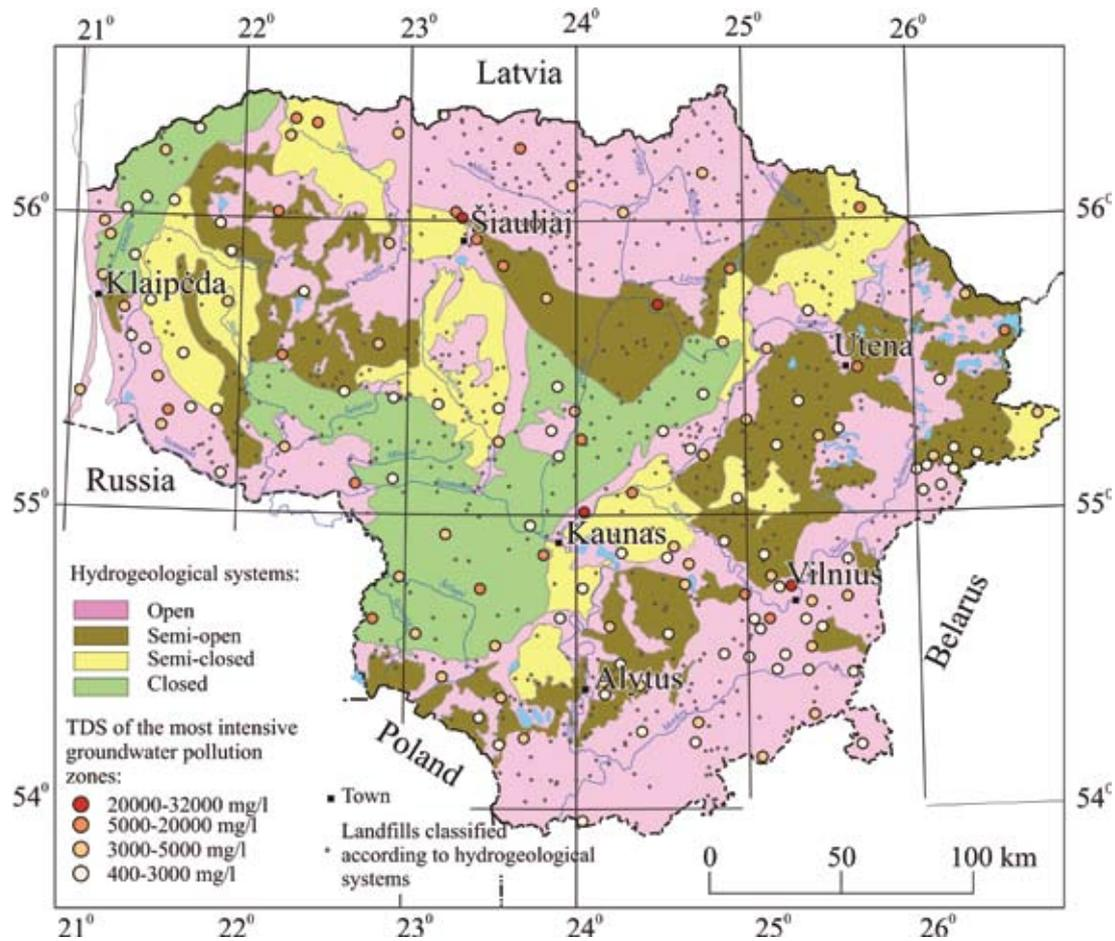
Fig. 4 Classification map of Lithuanian municipal waste landfills. Hydrogeological systems boundaries by Baltrūnas *et al.* 1998.
