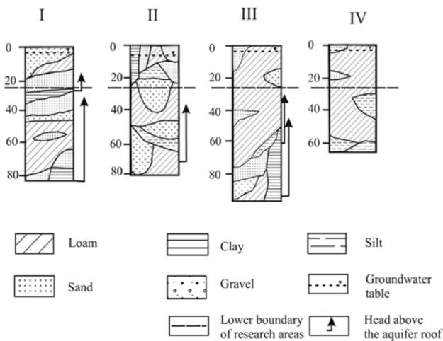
Fig. 2 Types of hydrogeological systems: I – open, simple filtration; II – semi-open, complex filtration; III – semi-closed, complex filtration; IV – closed, highly complex filtration. Hydrogeological profiles by Baltrūnas et al. 1998
