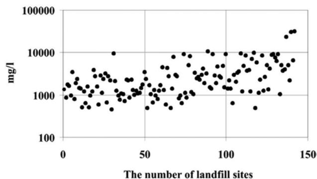
**Fig. 6** The distribution of average TDS concentration values in the most intensive groundwater pollution zones in 142 landfill sites
