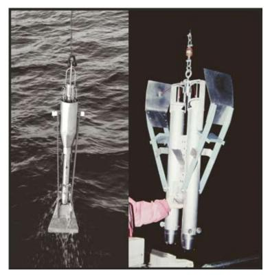
Fig. 1 The *Niemistö* and *Gemini* corers used during geochemistry studies of the GTK. Photos by Henry Vallius
