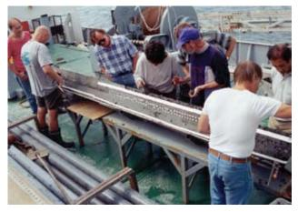
**Fig. 5** Subsampling of a *Kastenlot* core during a BASYS Subproject-7 cruise on board R/V *Petr Kottsov*. The cubes for palaeomagnetic dating are well visible in the sediment surface. Photo: Henry Vallius
