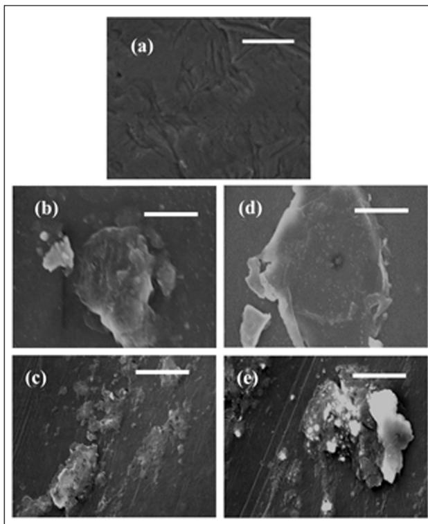
**Fig. 3.** Comparative SEM micrographs of PVC film degraded by consortium CP-I (b and c) and CP-II (d and e) before and after formulation in talc, respectively, by taking untreated PVC film as control (a). Scale bars = 10 µm; magnification = 3.00 KX
