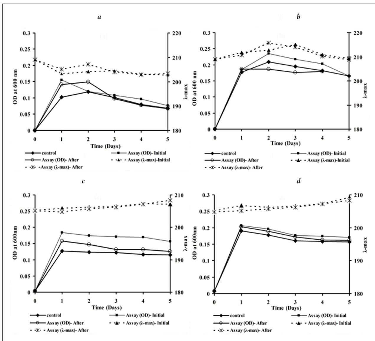
Fig. 1. Comparative *in vitro* biodegradation assay of LDPE film using consortium H (a), consortium L (b) and PVC film using consortium CP-I (c), consortium CP-II (d) before and after retrieval from talc based formulation
