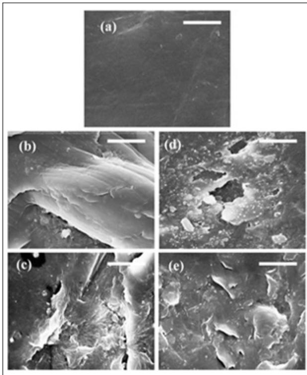
**Fig. 2.** Comparative SEM micrographs of LDPE film degraded by consortium H (b and c) and L (d and e) before and after formulation in talc, respectively, by taking untreated LDPE film as control (a). Scale bars = 10 µm; magnification = 3.00 KX
