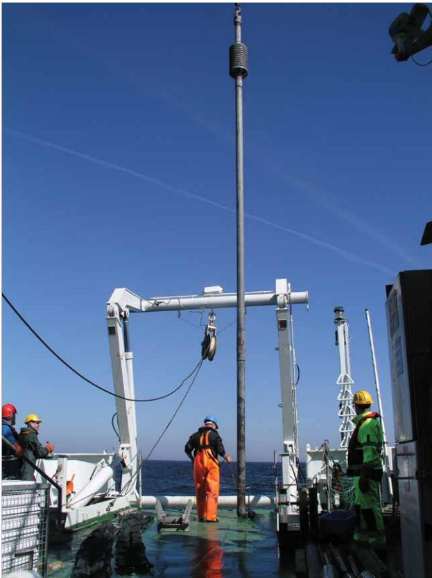
Fig. 2 Long gravity corer (IOW, 9 m) in use onboard R/V Aranda during INFLOW cruise in the Gotland basin. Photo by A. Kotilainen, April 2009.
