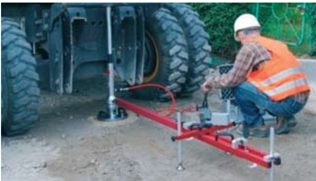
Fig. 2 Static plate load test ( https://www.hmp-online.com )
