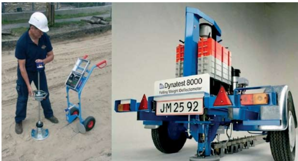
Fig. 1 On the left side – dynamic plate, on the right – a falling weight deflectometer ( https://www.dynatest.com/ )
