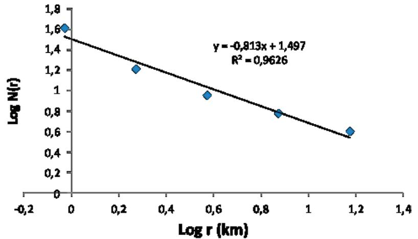
Fig. 7 The smallest fractal dimension value was obtained for the boxed area of Hazar Lake and its surroundings. The manual version of the box counting method was applied
