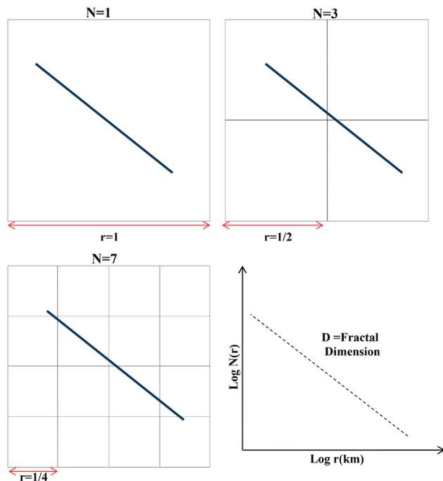
**Fig. 3** Simplified representation of the box counting method application (Aydındağ et al. 2018)
