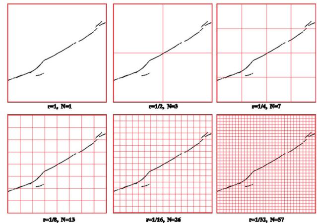
**Fig. 4** The manual (classic) application of the box counting method
