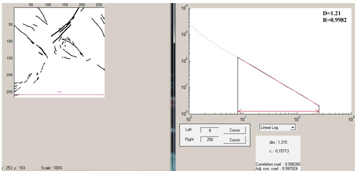
Fig. 10 The Free box method application (Bingöl-Center)
