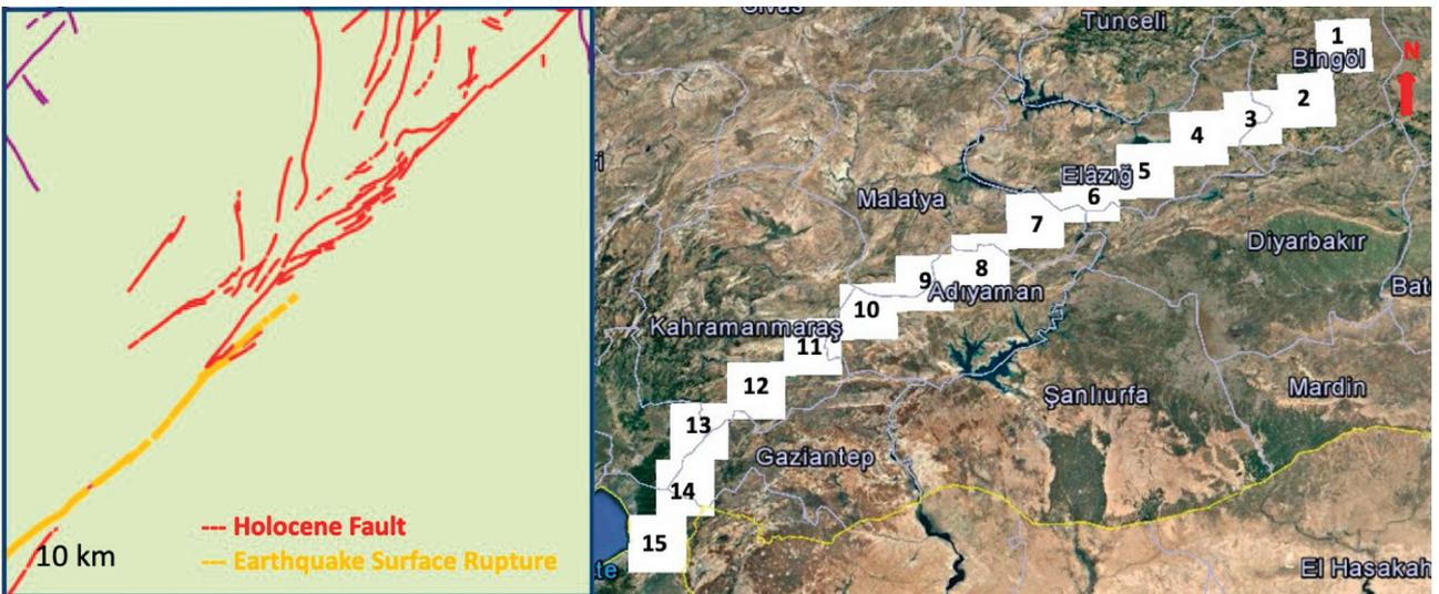
**Fig. 2** The Google Earth image showing the boxed segments along the East Anatolian Fault Zone (EAFZ) (based on the website of the General Directorate of Mineral Research and Exploration)
