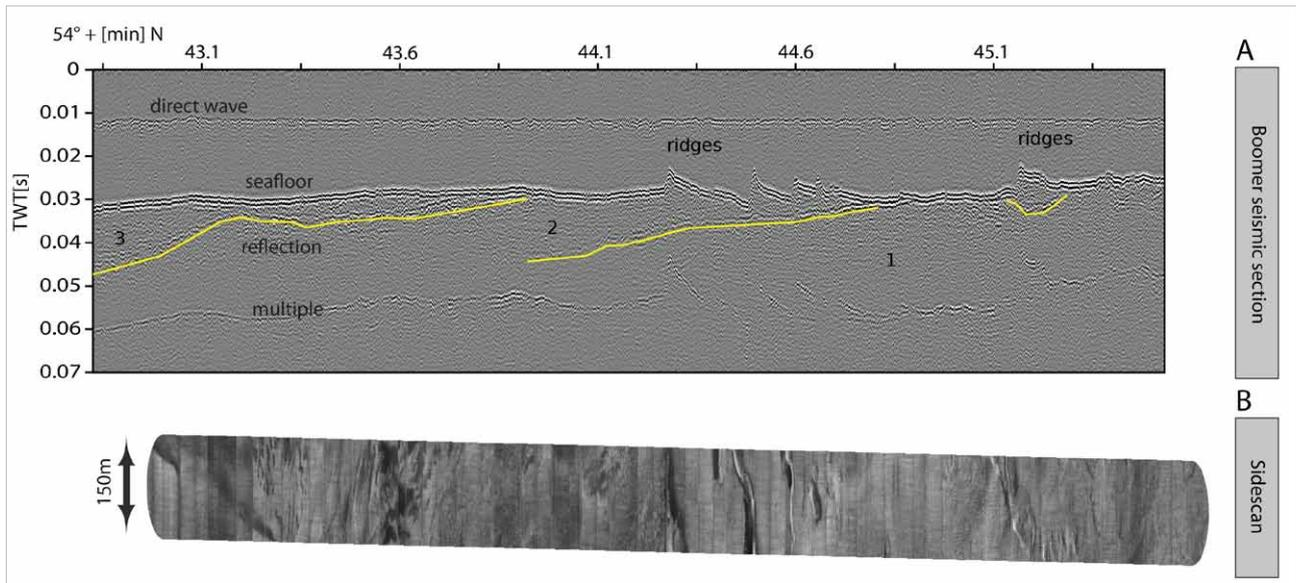
**Fig. 5** Profile 29, crossing the observed ridge system in North-South direction. Boomer data (A) and corresponding side scan sonar data (B) are displayed. Refer to Fig. 3 for position. Seismic units are indicated by numbers 1 to 3. Compiled by D. Wilken, 2013.
