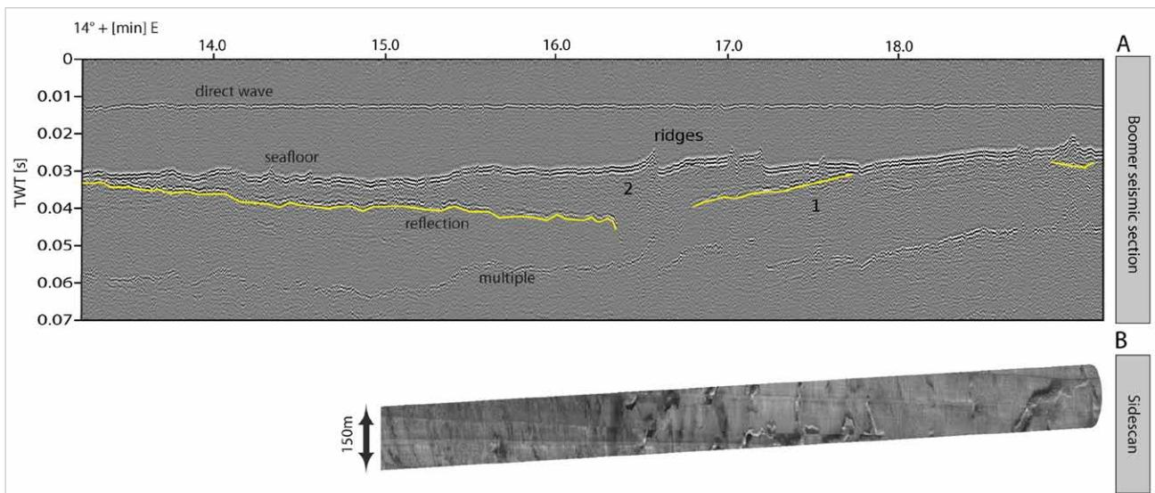
**Fig. 4** Profile 28, crossing the observed ridge system in East-West direction. Boomer data (A) and corresponding side scan sonar data (B) are displayed. Refer to Fig. 3 for position. Seismic units are indicated by numbers 1 to 3. Compiled by D. Wilken, 2013.
