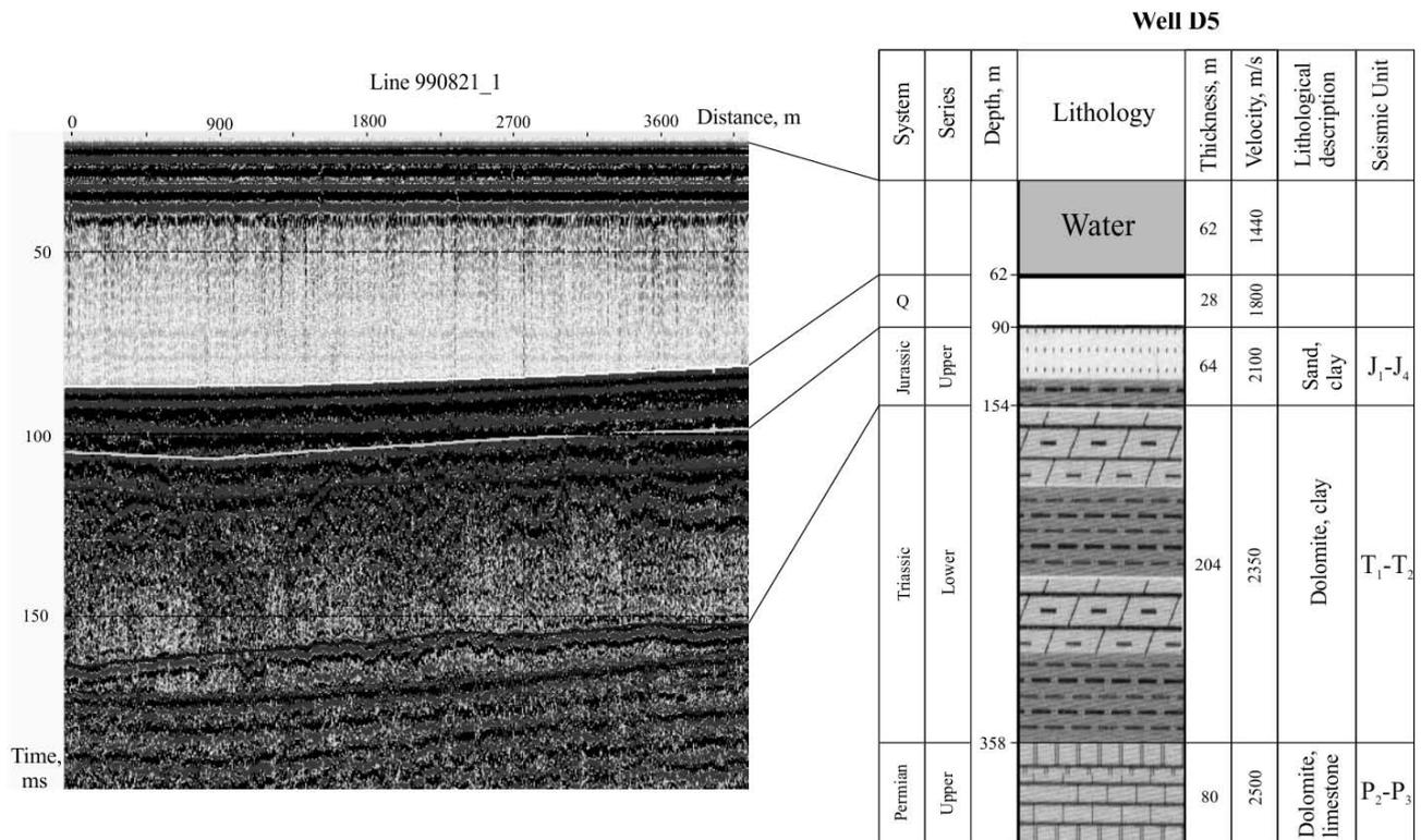
**Fig. 4** Basic seismic profile of the Quaternary–Permian sequence calibrated with D5 well data.
