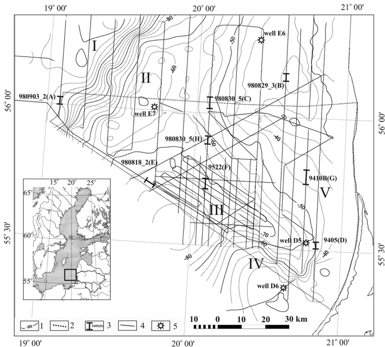
**Fig. 1** Location map: 1 – contour intervals at 5 m depth are drawn after seismoacoustic data; 2 – Lithuanian Sea border; 3 – fragments of seismic lines (see Fig. 5); 4 – seismic lines; 5 – wells. Morphology: I – eastern slope of Gotland Depression; II – Klaipėda–Ventspils Plateau (Klaipėda Bank and Liepaja Bank); III – northern part of Gdansk Depression and its Klaipėda Slope; IV – Curonian Plateau; V – near shore zone.
