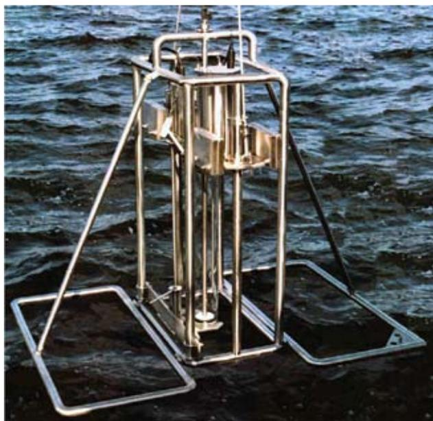
**Fig. 11** The OSCOR corer being deployed over board. Upon contact with the bottom a battery driven electric motor causes the core barrel to quickly rotate (oscillate) back and forth aiding the clear plastic core barrel to penetrate into sandy sediment. Photo courtesy by Cees Laban
