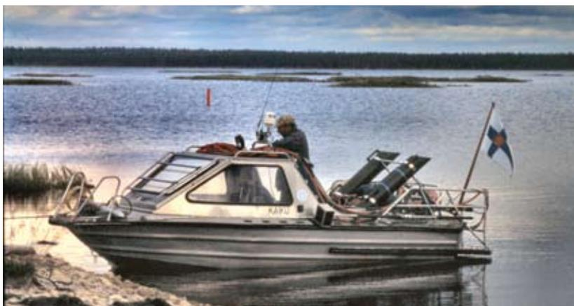
**Fig. 12** The *Kaiku* (=Echo) motorboat was fully equipped with Meridata’s MDPS-integrated GPS-positioning, echo-sounder, side scan sonar and single channel low frequency towed profiler with hydrophone streamer for wide band acoustics with excellent penetration in sand, gravel and till. Electronics engineer Matti Tuhkanen is the main operator of the boat and its data acquisition equipment
