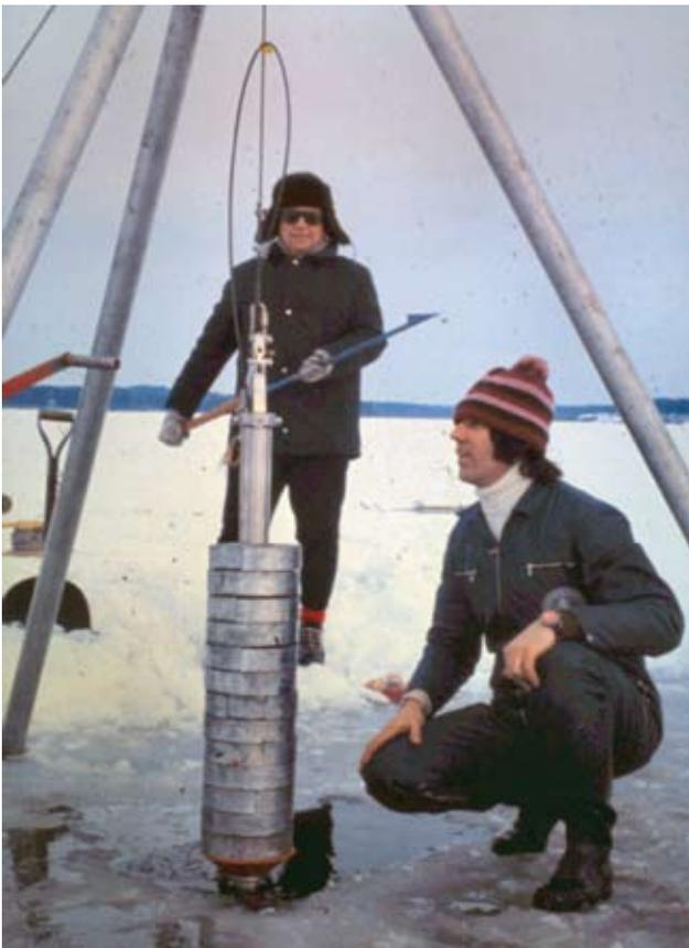
**Fig. 7** Although the piston corer was originally designed for marine sediment sampling it is just as suitable for wintertime coring in deep lakes or even coastal lagoons not reachable by boat. Heikki Ignatius in the background with icepick in his hands although the hole in the ice was made with a long chainsaw. Technician Pauli Kaijola is checking the lead weights. Photo taken by B. Winterhalter 50 years ago in Finnish Lapland
