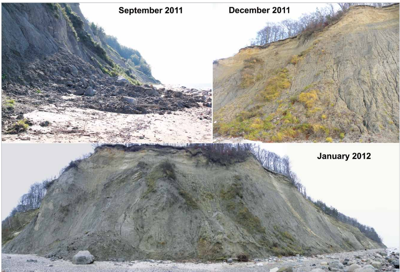
Fig. 5 Czubiński Reserve (CzR) test site during the research periods May 2011 – May 2012. Visible rockfall, slope wash and a system of erosion rills. Photos were taken in December 2011 and January 2012 from roughly the same point of view. Photos by R. Kolander.
