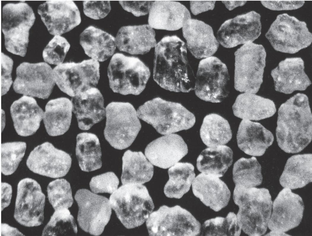
**Fig. 2.** Image of wind-blown sand with a diameter of 0.2-0.1 mm made by optic microscope
