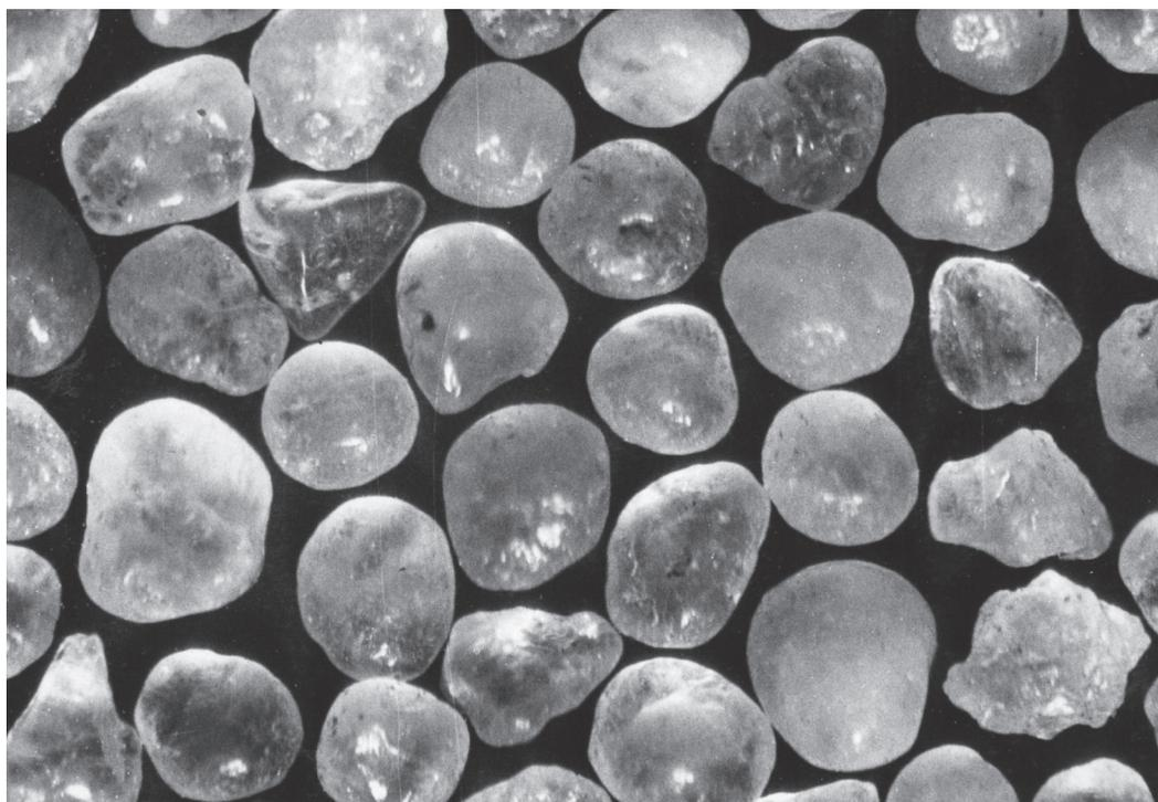
**Fig. 1.** Sand with a diameter of 0.63–1.0 mm of the Bug River at Zegerz (North of Warsaw)
