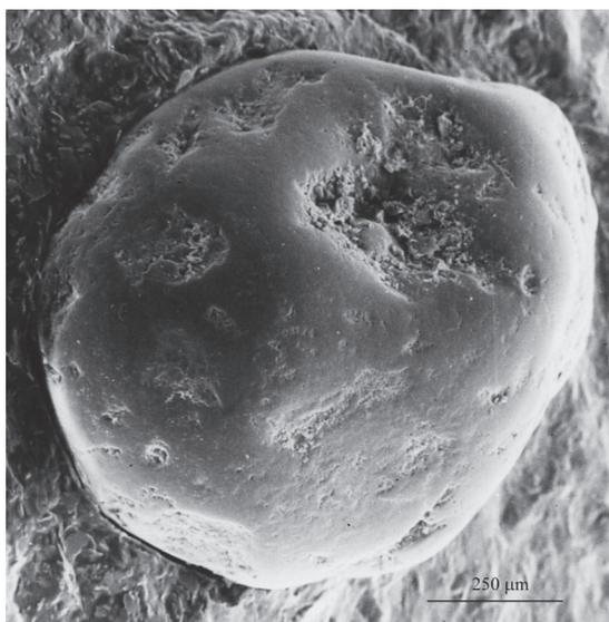
**Fig. 9.** Well rounded sand grain from shore environment. Solution marks are visible on the surface of the grain originating from a depth of 535 m
