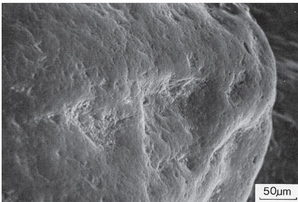
**Fig. 11.** Part of the surface of a wind-blown sand grains. Breaking steps characteristic of fluvial sand are still well observable at places (Jánoshalma 18)
