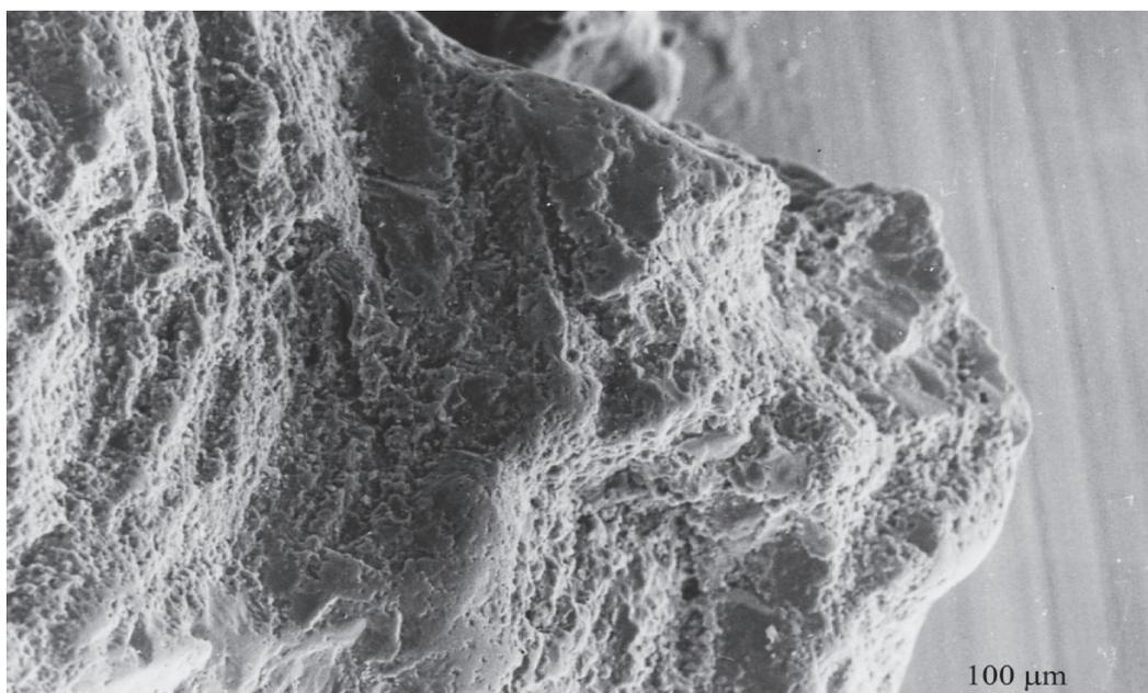
**Fig. 8.** Fluvial sand grain with solution marks taken from a depth of 480 m
