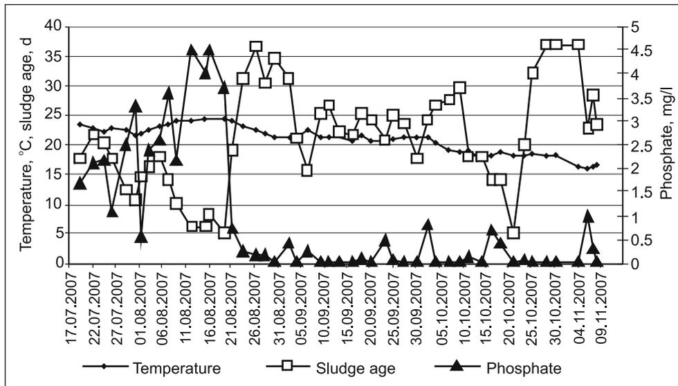
Fig. 1. Dynamics of phosphate in the aeration zone, sludge age and temperature
