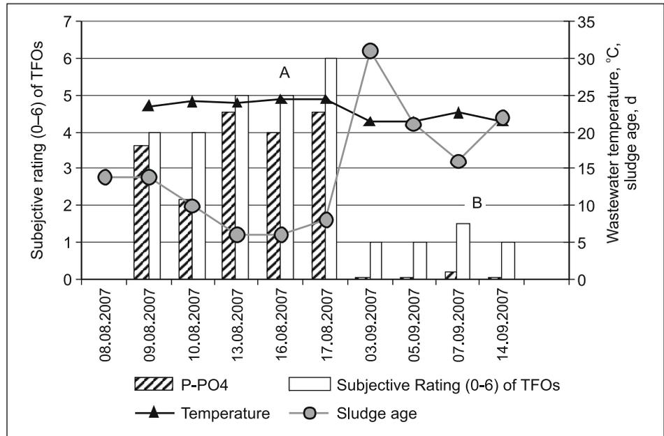
Fig. 3. Comparison of TFO populations in samples from A and B
