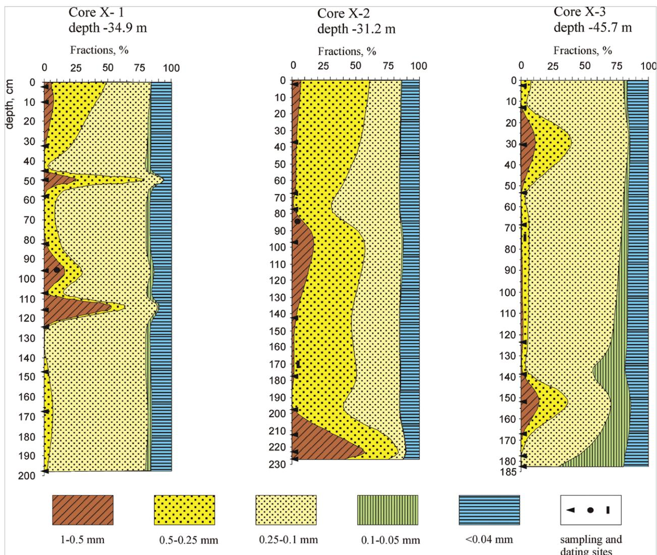
Fig. 5. Grain size composition, cores X-1, X-2, X-3.
