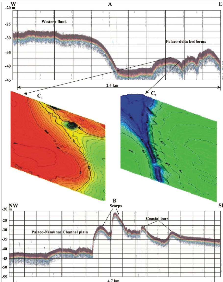
Fig. 2. Topography profiles A, B, C across the Palaeo-Nemunas delta. C<sub>1</sub> and C<sub>2</sub> show the palaeo-delta bed forms.
